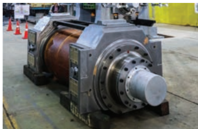
Shop assembly of 6-Hi Mill
